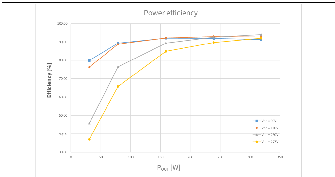
Figure 16 ICL5102 320 W reference board power efficiency measurement
