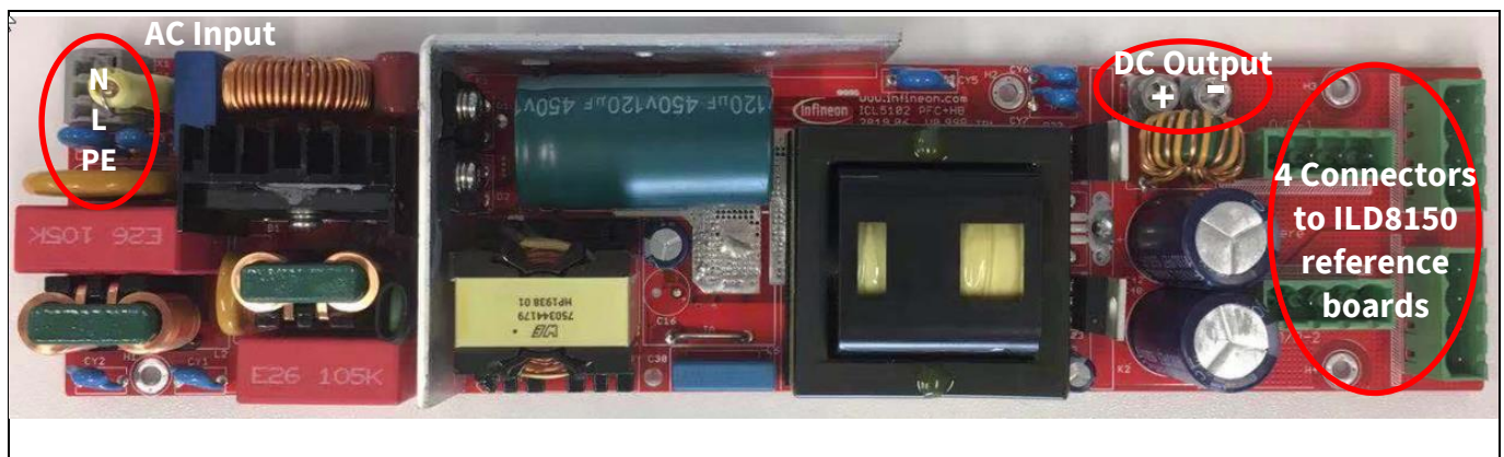
Figure 1 ICL5102 320 W CV reference board – top side
