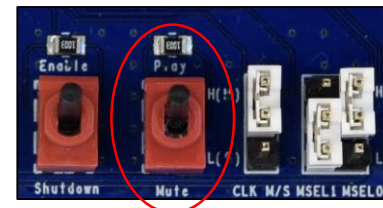
Figure 11. Right toggle switch set to “play” position.
