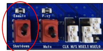
Figure 8. Left toggle switch set to “enable” position.
