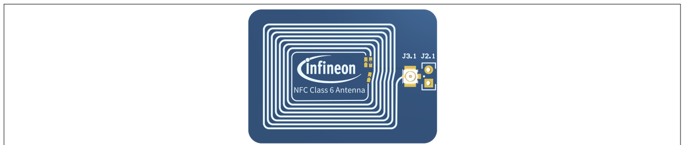
Figure 7 Class 6 shield antenna in its default configuration (usage with the included UMCC cable)
