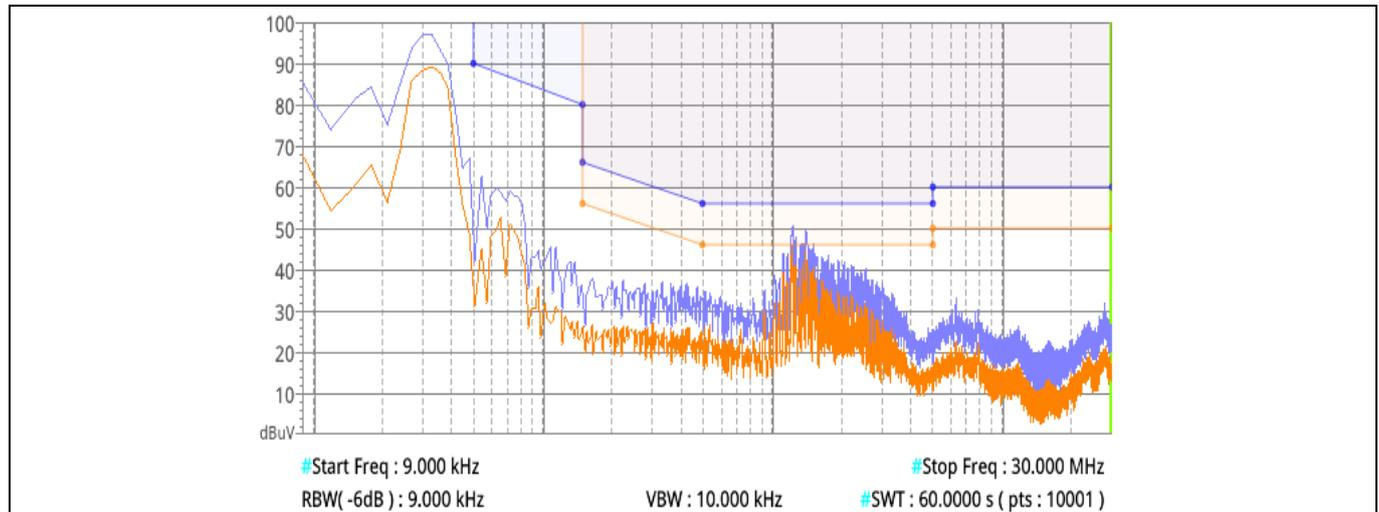
**Figure 15** IPD90R1K2C3 EMI test result with EN 55015 limits
