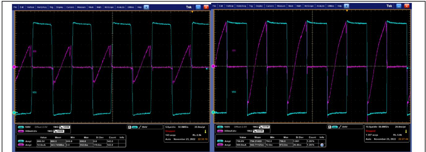
**Figure 11** IPD95R450PFD7 drain-to-source voltage and drain current waveforms at  $V_{out} = 17\text{ V}$   $P_{out} = 0\text{ W}$  on the left,  $P_{out} = 52\text{ W}$  on the right
