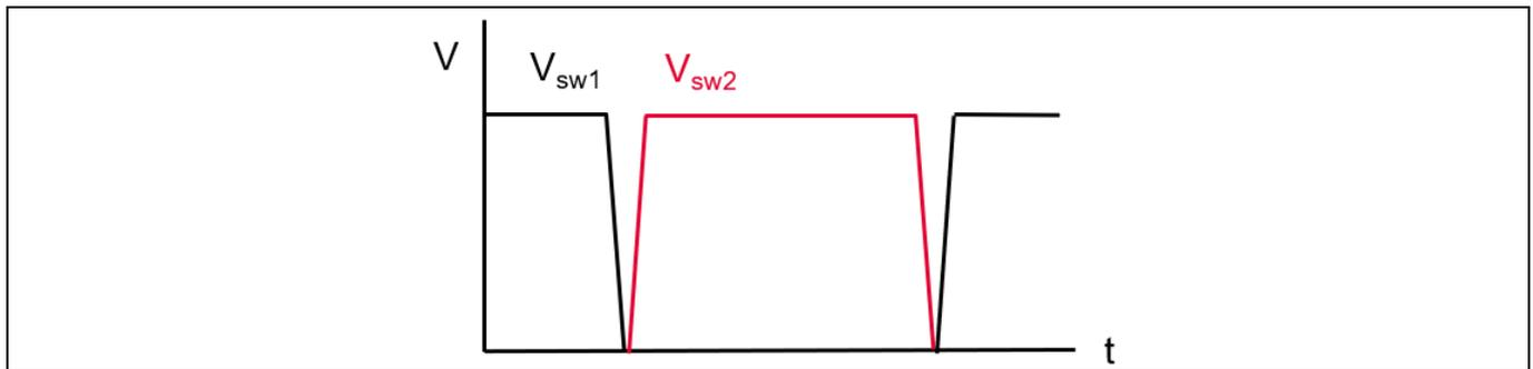
**Figure 5** Simplified drain-to-source voltage waveforms in LCC
