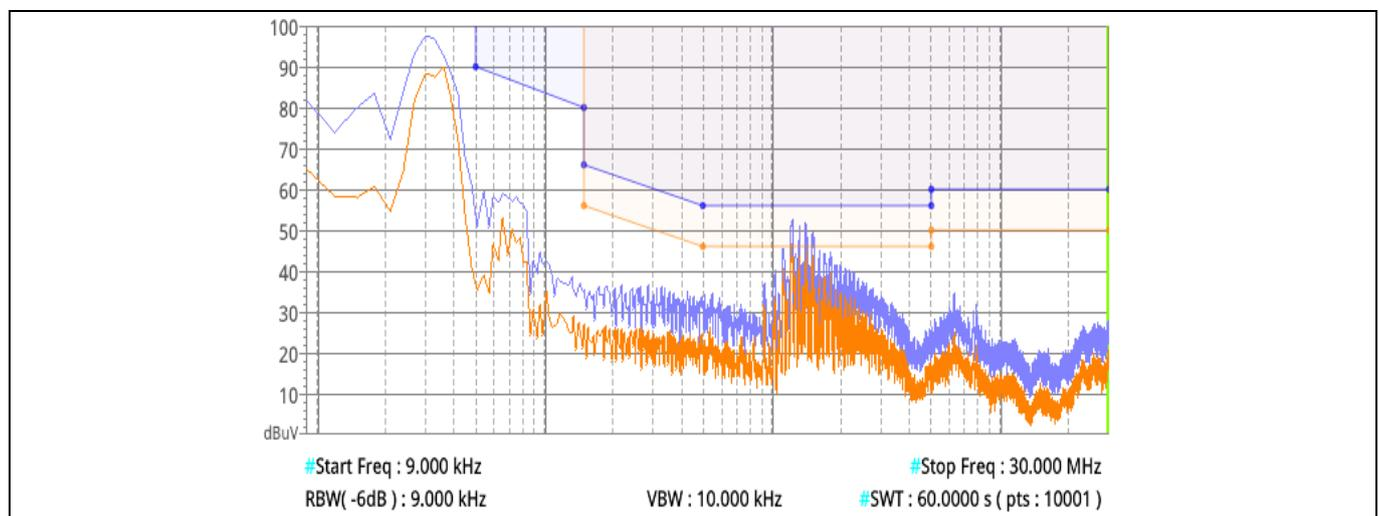
**Figure 16** IPD95R450PFD7 EMI test result with EN 55015 limits
