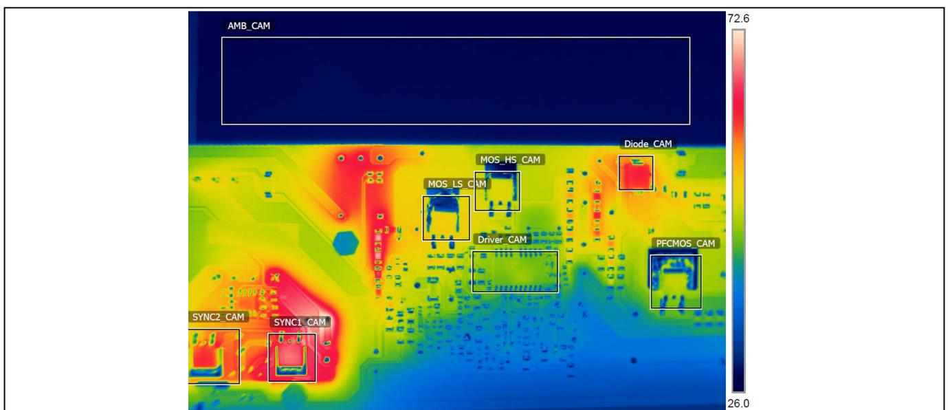
**Figure 14** Board backside thermal image at 48 V 3 A output with IPD95R450PFD7
