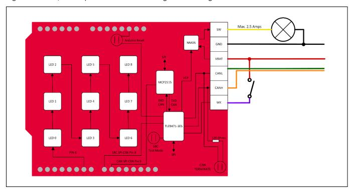
All CAN communication is done on 500 kBaud/s bus speed. After start-up, following features can be used:
