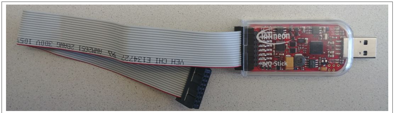
Figure 31 Infineon \mu IO-Stick with ribbon cable
