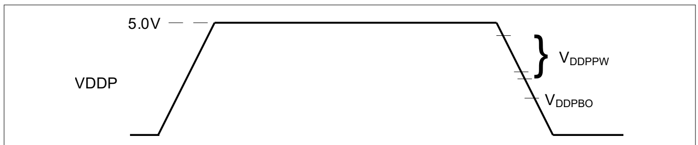
Figure 11 Supply Threshold Parameters
