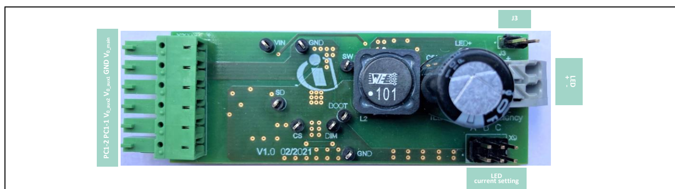
Figure 7 Reference design – dimensions 81 mm (L) x 27 mm (W) x 24 mm (H)
