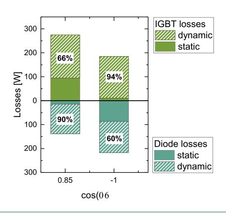
Power losses ratio for the FF600R17ME4\_B11 under the following conditions:
