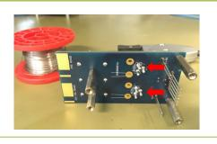
Step 2 Source resistor soldering
