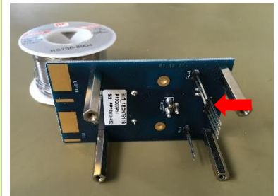
Step 4 TO-220 socket soldering
