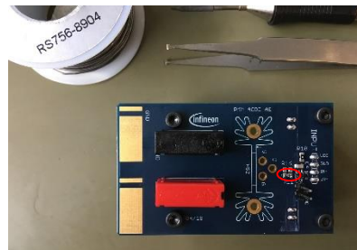
Step 5 MOSFET placement into the socket
