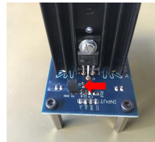
Step 7 IN- jumper connection
