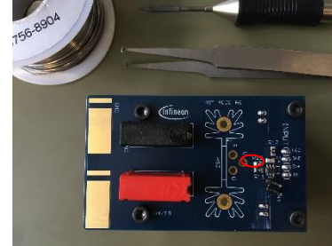
Step 7 IN- jumper connection
