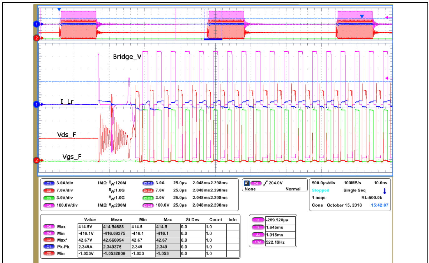
Figure 23 Burst operation with pre-charge of bootstrapping capacitors
