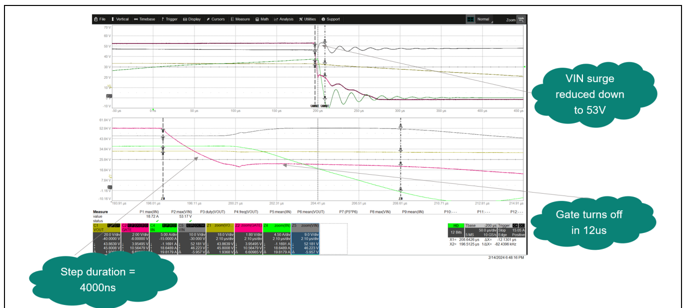
Figure 43 Two-step shutdown to turn off MOSFET after SOC fault
