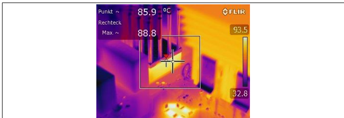
Figure 32 Thermal image of the input rectifier
