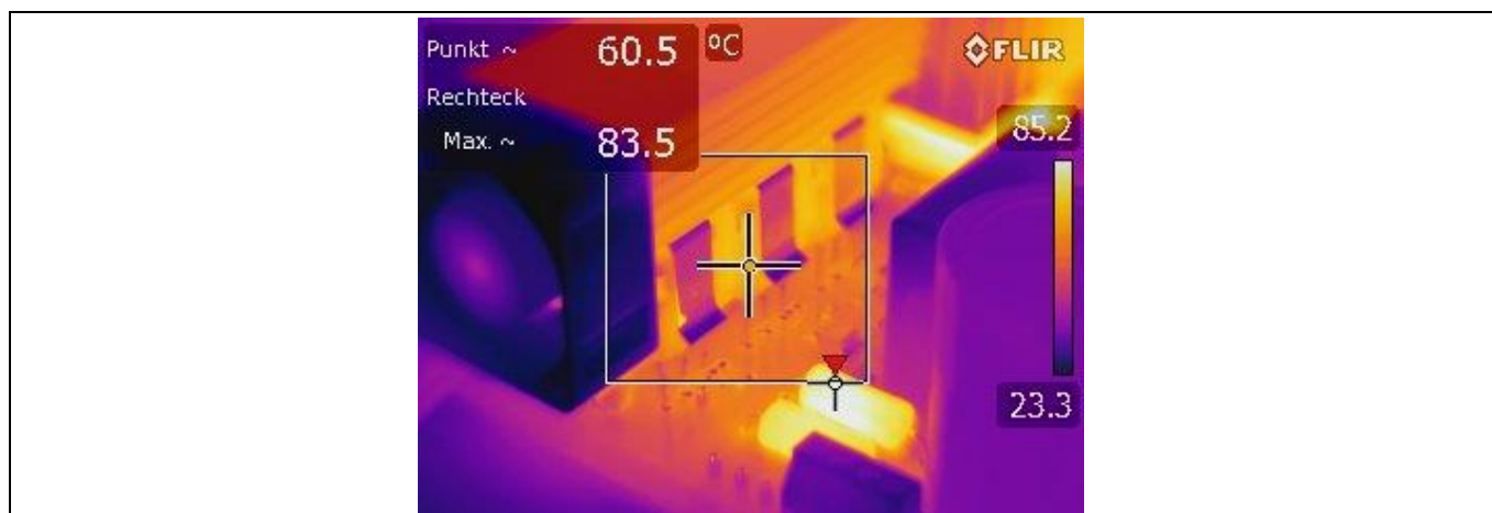
Figure 34 Thermal image of evaluation board at 18 kHz switching frequency, 10 Ω gate resistance and forced convection
