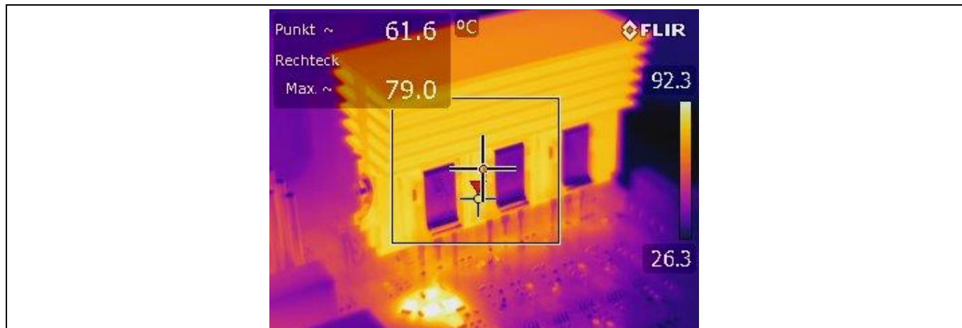
Figure 30 Thermal image the left power MOSFETs
