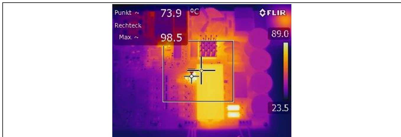
Figure 33 Top view thermal image (hotspot at voltage measurement resistors)
