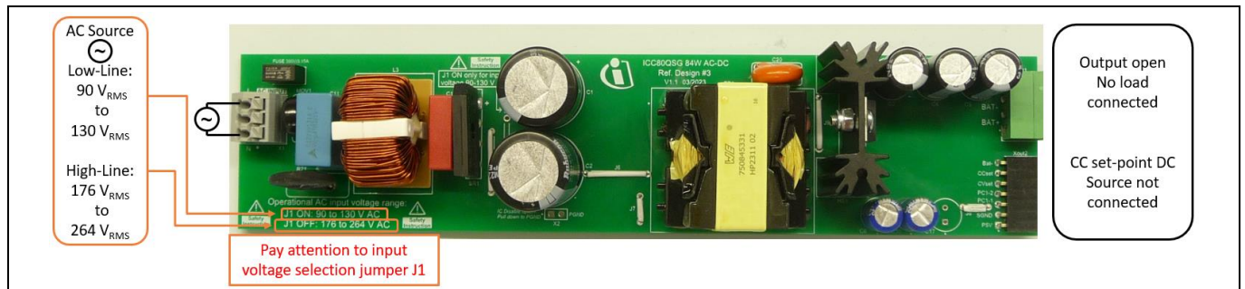
Figure 4 No-load system standby power test setup
