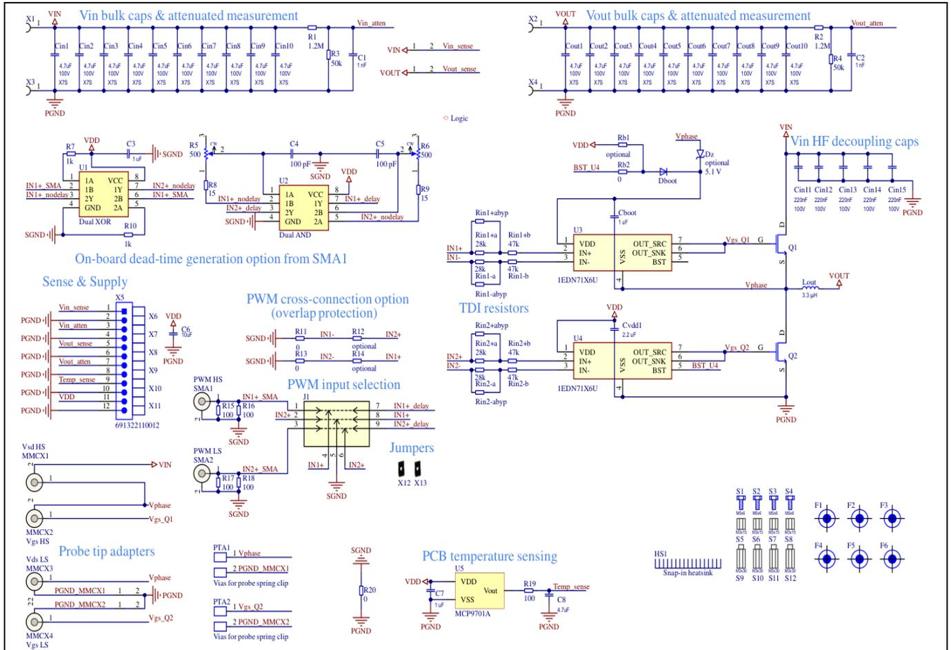
Figure 38 EVAL\_7136U\_100V\_GaNc schematic
