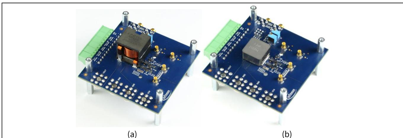
**Figure 12 (a) Mounted inductors - TDK ERU series and (b) Vishay IHLP7575-JZ series**
