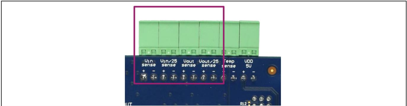
**Figure 13** Screw terminal plugs for DC voltage measurement
