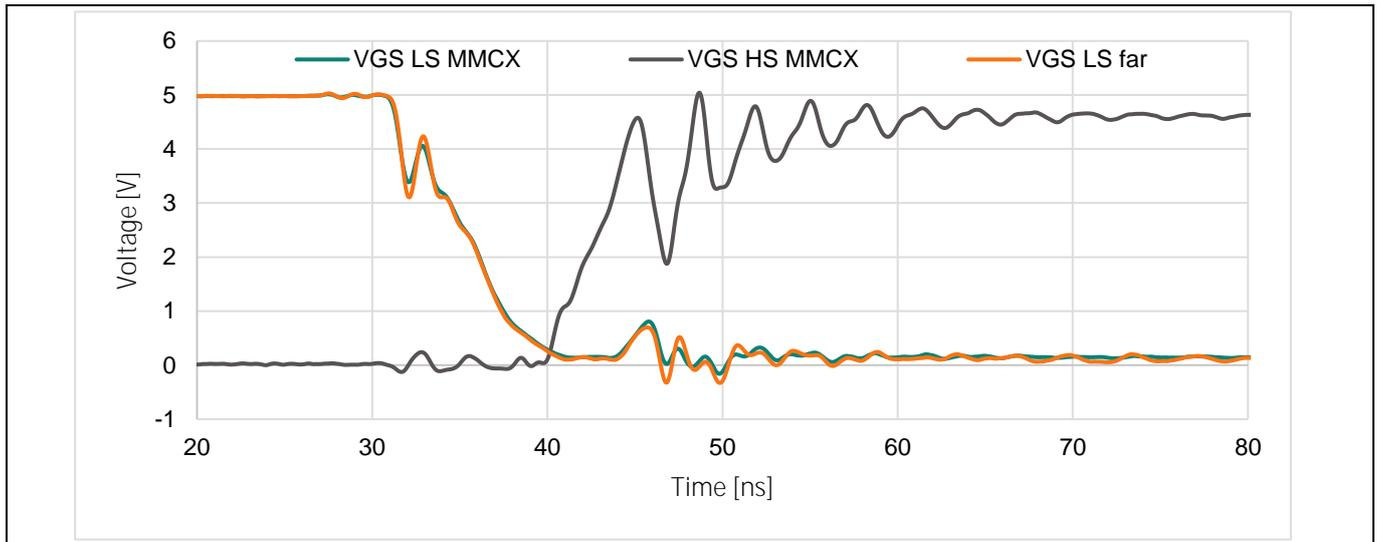
Figure 28 Buck-mode example waveforms - turn on gate voltages
