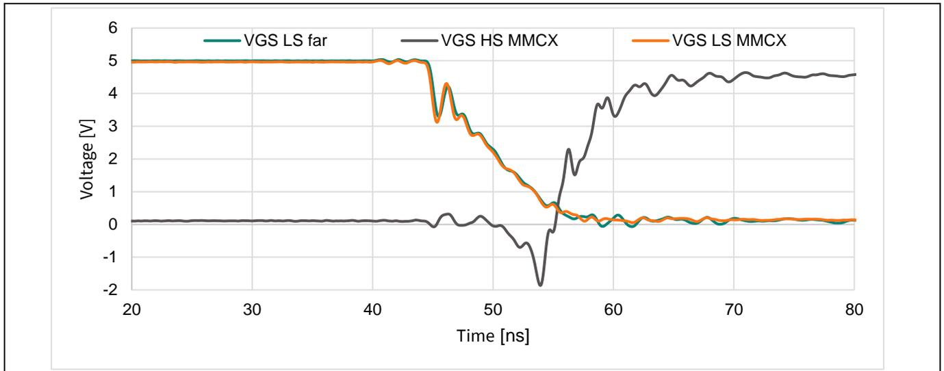
**Figure 30** Boost-mode example waveforms - turn off gate voltages
