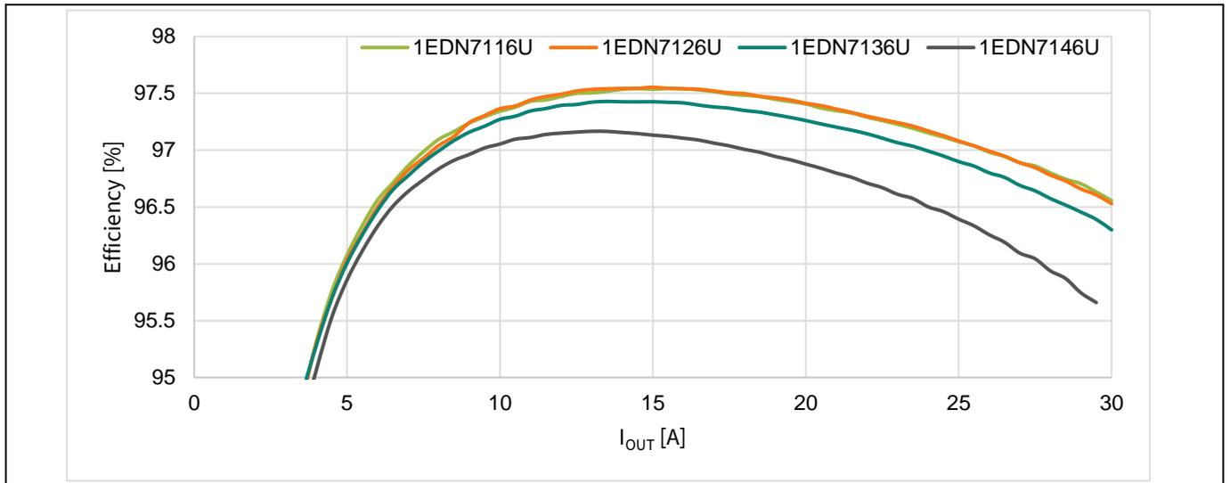
Figure 35 Buck-mode example efficiency results for all four gate driver variants
