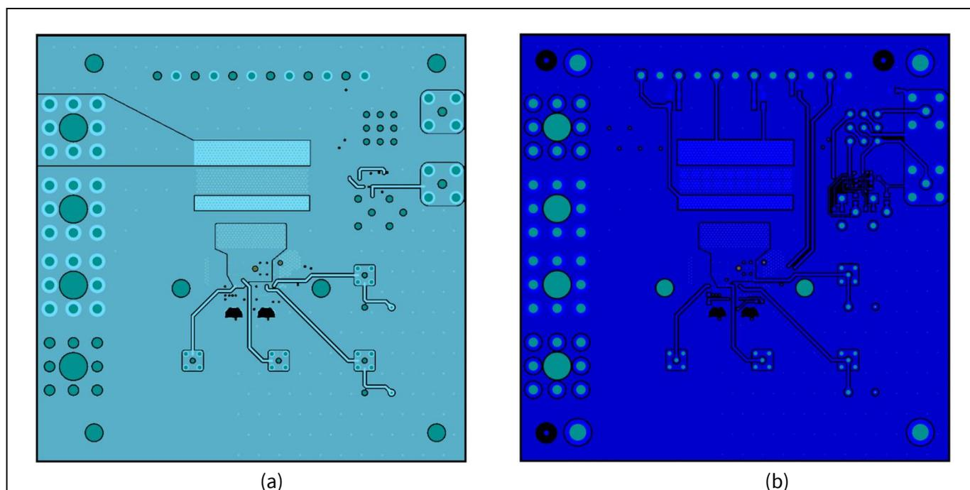
Figure 40 (a) PCB layout mid-layer 2 and (b) bottom layer
