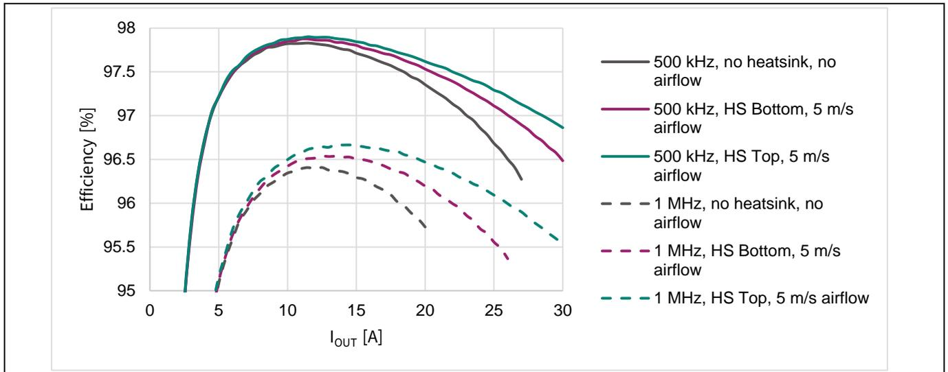
**Figure 22** Example efficiency results with TDK ERU 10  $\mu$ H inductor
