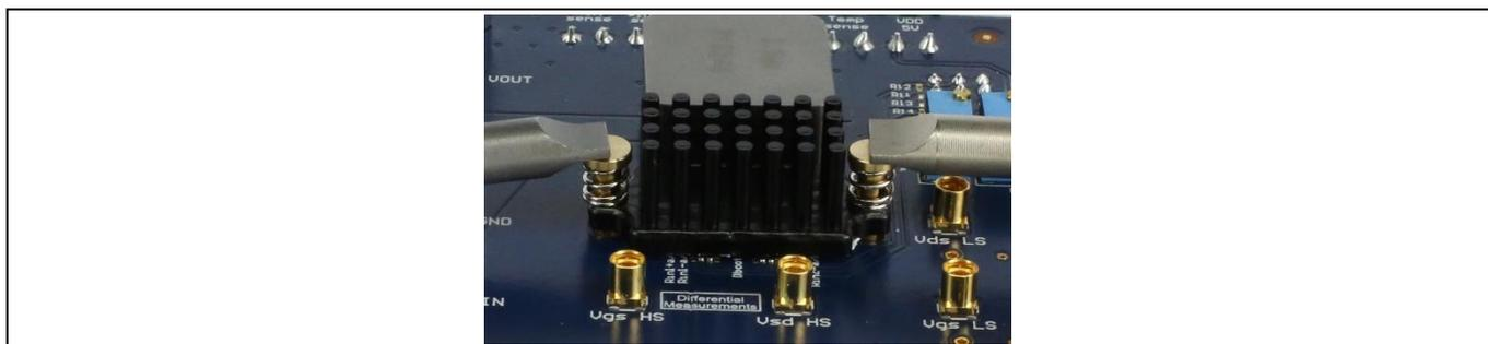
**Figure 11 Heatsink attachment with two flathead screwdrivers to compress spring pins**
