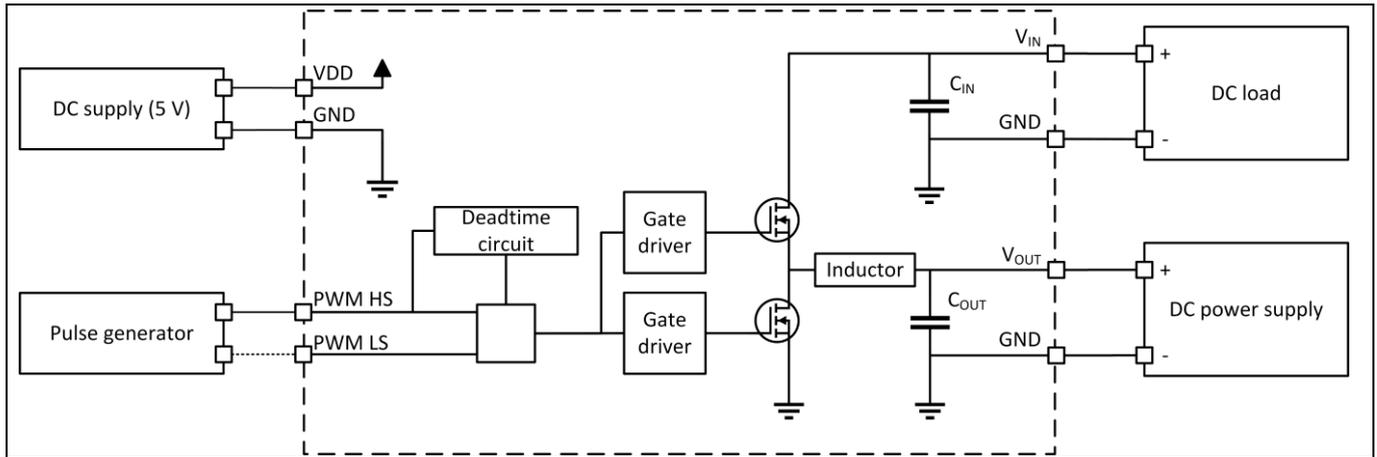
**Figure 5** Block diagram of boost converter test setup
