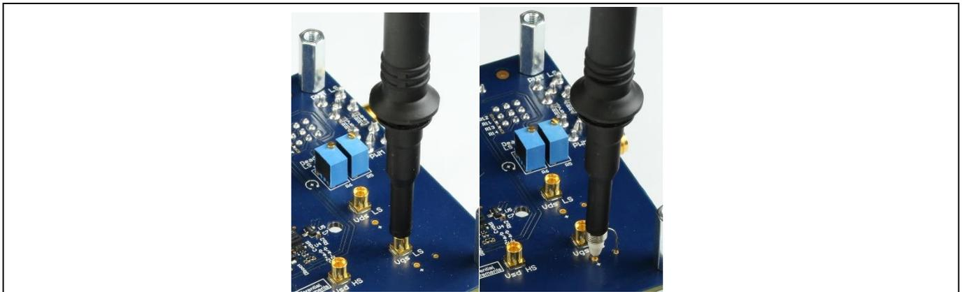
**Figure 15** Low-side single ended voltage measurements options
