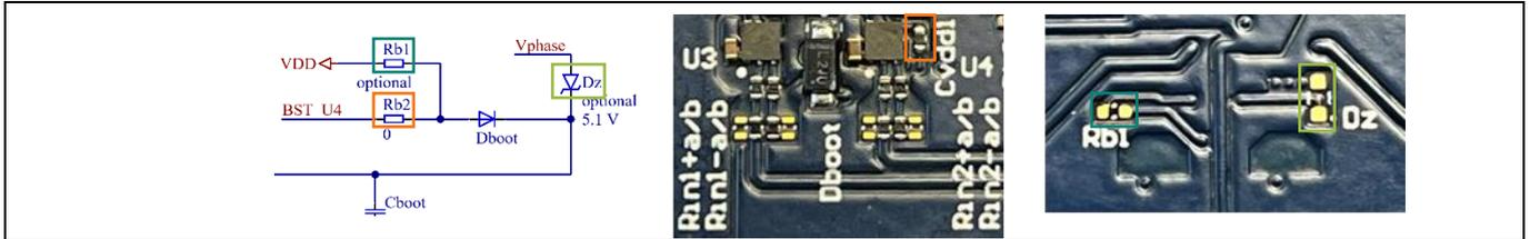
**Figure 20** Rework instructions for conventional bootstrapping from V<sub>DD</sub>
