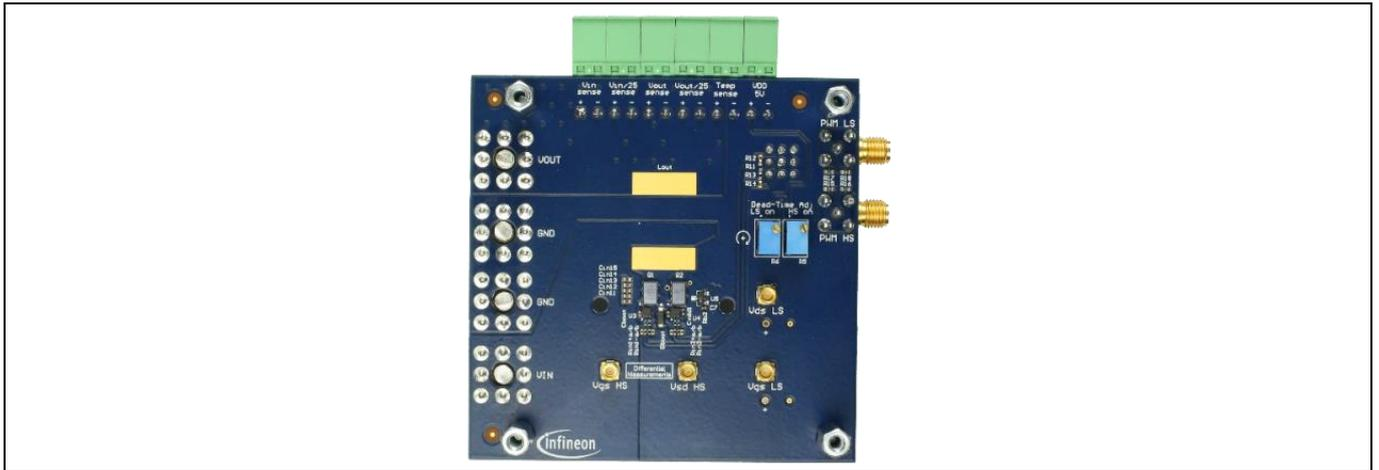
**Figure 1** EVAL\_7136U\_100V\_GaNc Evaluation Board
