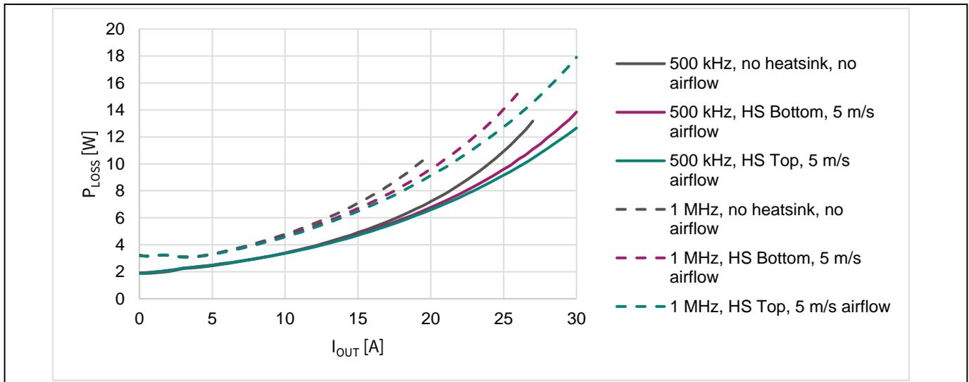
**Figure 25** Example power loss results with Vishay IHL7575-JZ 3.3 μH inductor
