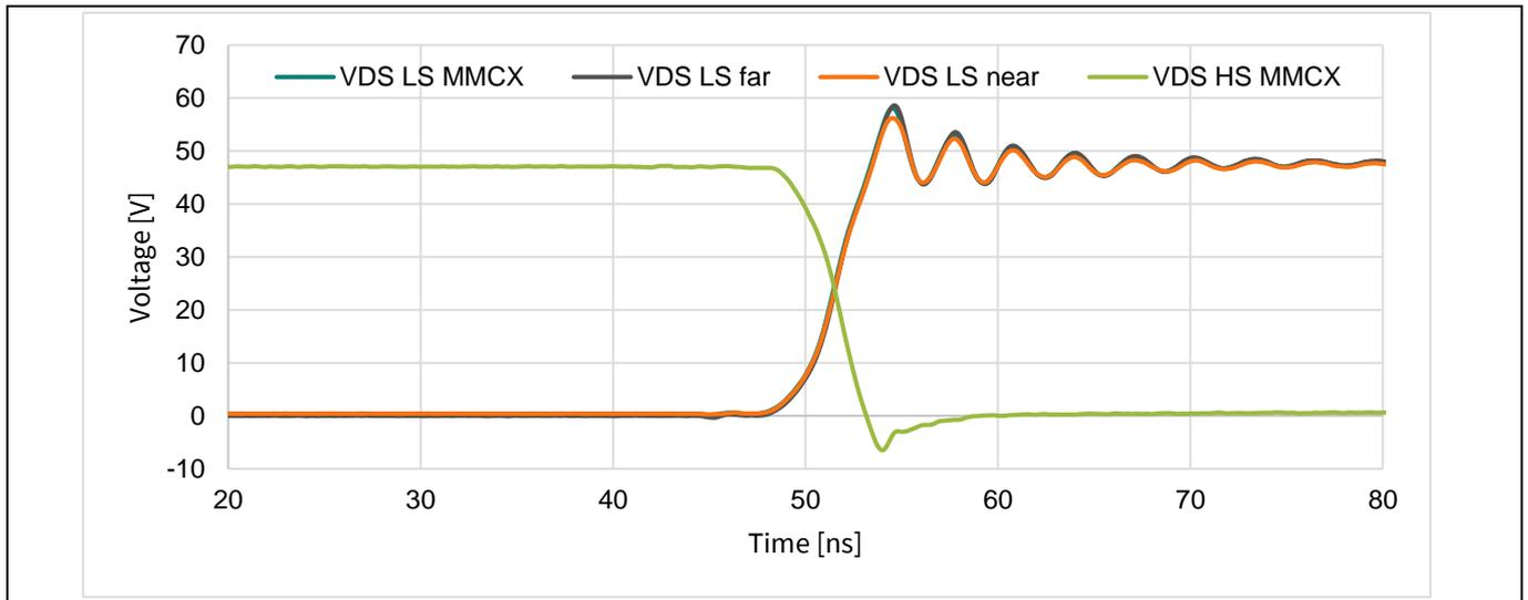
**Figure 31** Boost-mode example waveforms - turn-off drain voltages
