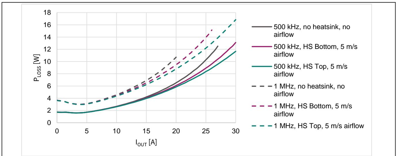
**Figure 23** Example power loss results with TDK ERU 10  $\mu$ H inductor
