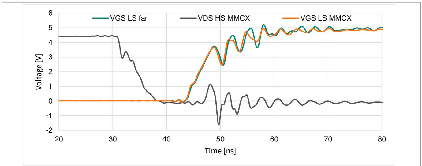
Figure 32 Boost-mode example waveforms - turn on gate voltages
