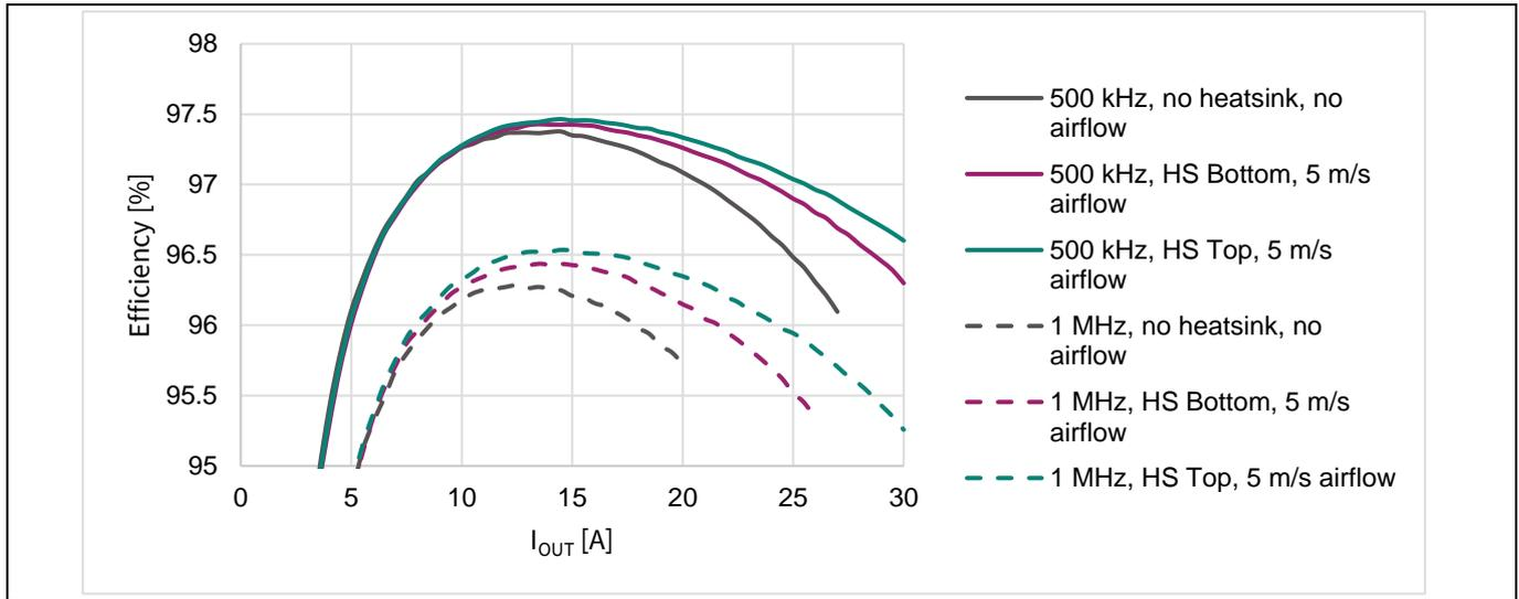
**Figure 24** Example efficiency results with Vishay IHL7575-JZ 3.3 μH inductor
