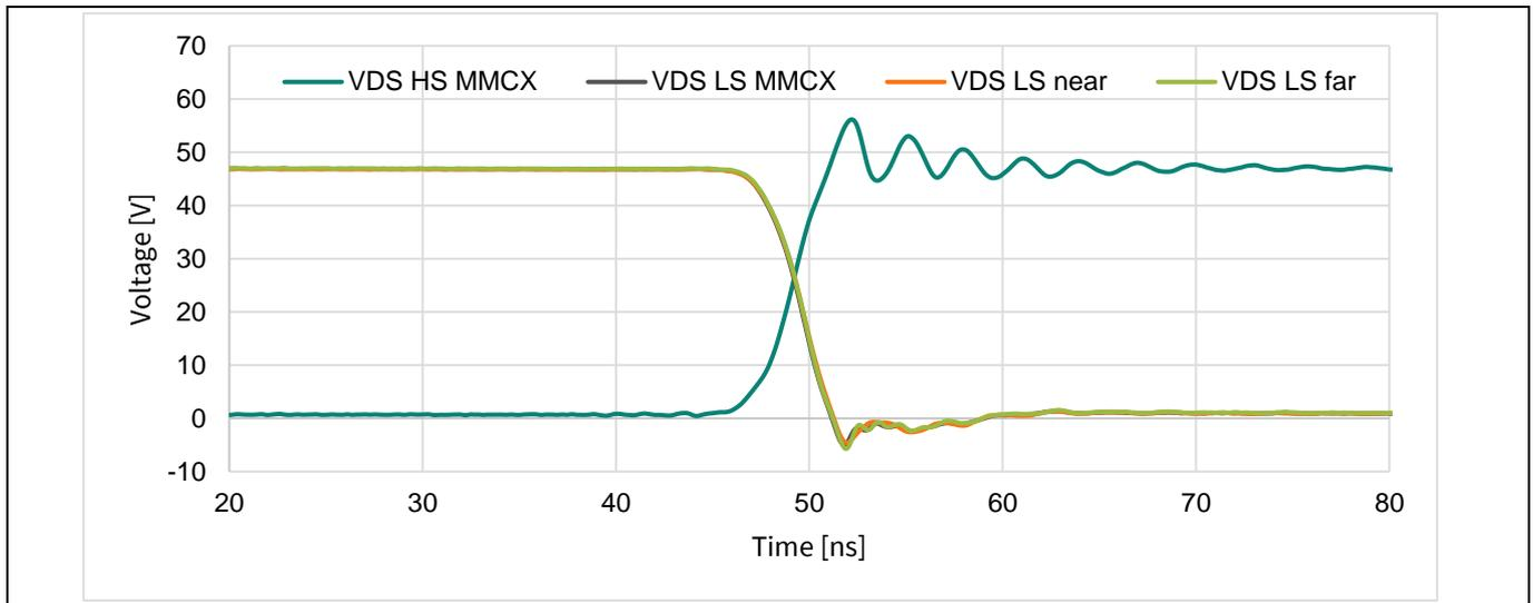
**Figure 27** Buck-mode example waveforms - drain voltages during high-side turn-off transition
