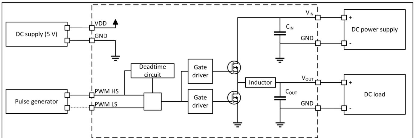
Figure 4 Block diagram of buck converter test setup
