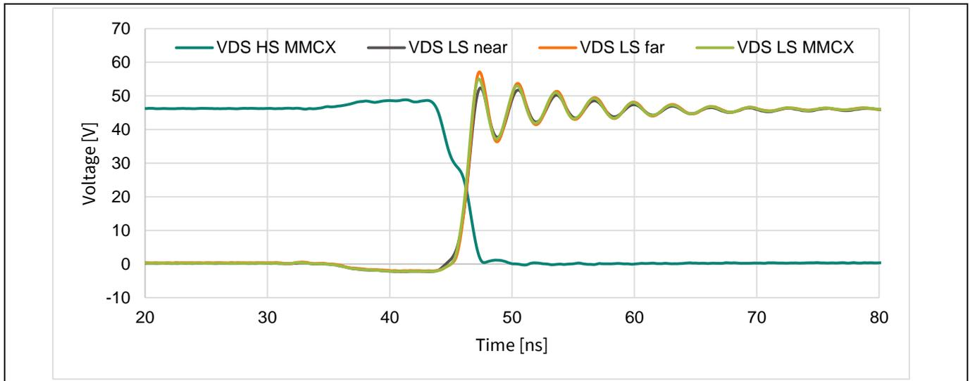
Figure 29 Buck-mode example waveforms - turn on drain voltages
