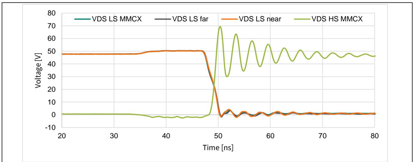
Figure 33 Boost-mode example waveforms - turn on drain voltages
