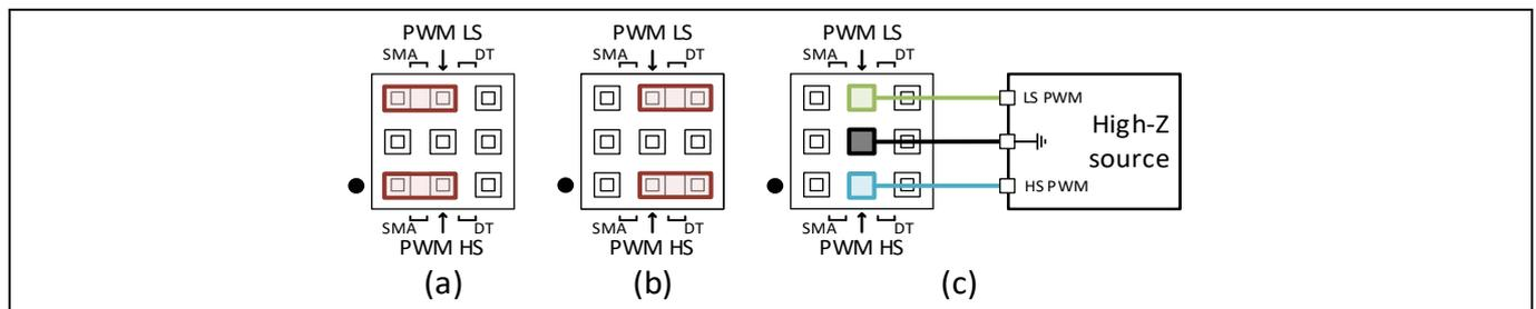
**Figure 8 (a) Jumper J1 settings for dual 50 Ω logic inputs, (b) single high-side 5 V logic input, and (c) dual 5 V high-Z terminated logic inputs**
