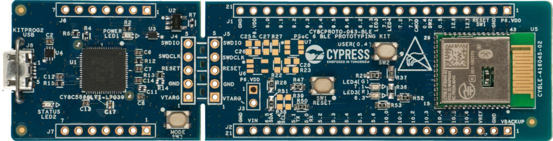
Figure 1-2. CY8CPROTO-063-BLE PSoC 6 Prototyping Board - Bottom View
