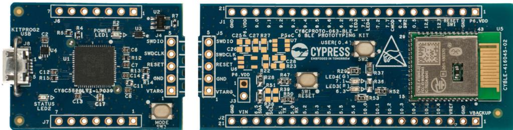
After the PSoC 6 BLE Prototyping Board is broken into two, the two halves can be reconnected for programming and debugging by adding connectors at J5 and J6. Also, a Cypress MiniProg3 device can be connected to a connector at J5 to perform programming and debug.
