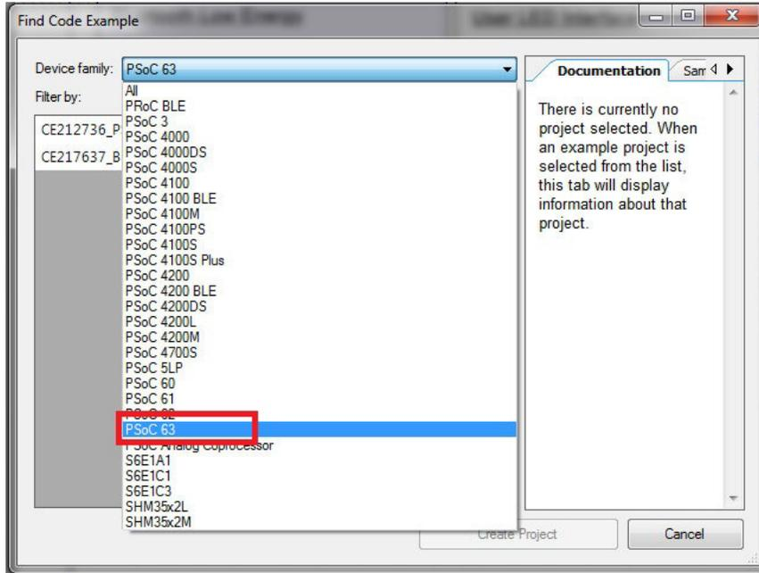
4. You can select the *CE217637\_BLE\_Find\_Me* project and see how to use it with the CY8CPROTO-063-BLE Prototyping Board.
