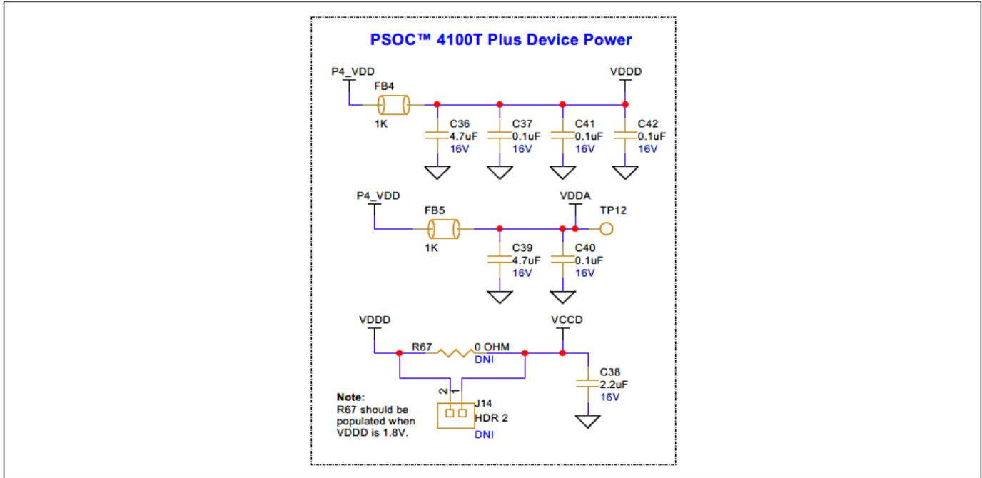
Figure 35 PSOC™ 4100T Plus device power schematic
