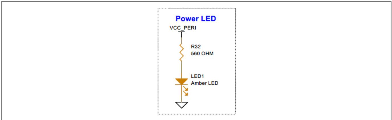
**Figure 25** Schematic of power LED indication (LED1)
