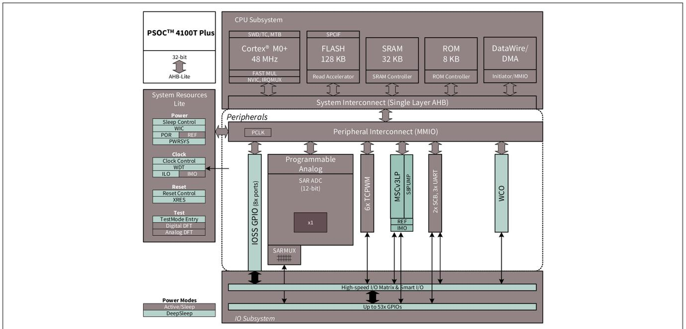
Figure 3 PSOC™ 4100T Plus device block diagram
