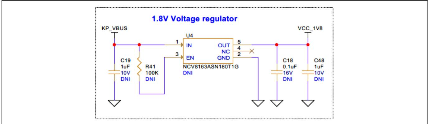
**Figure 33** 1.8 V voltage regulator (U4) schematic
