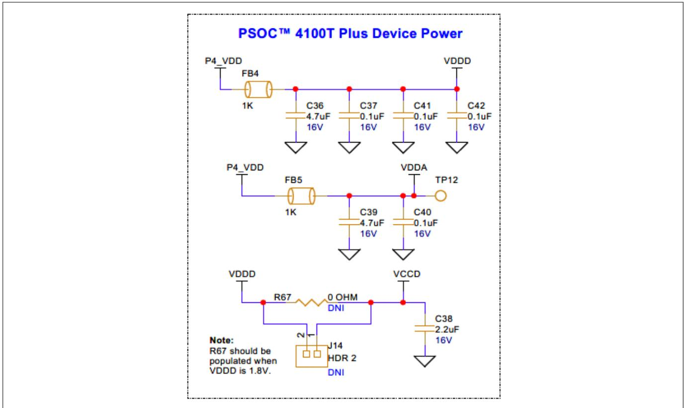
**Figure 22 PSOC™ 4100T Plus MCU power schematic**
