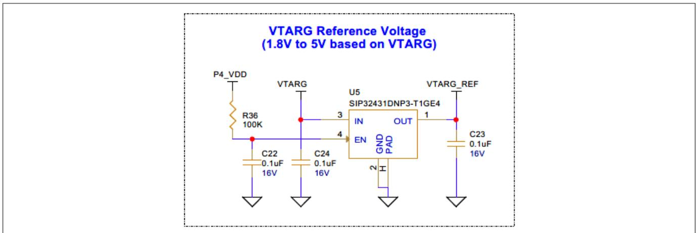
Figure 36 Target reference voltage switch (U5) schematic
