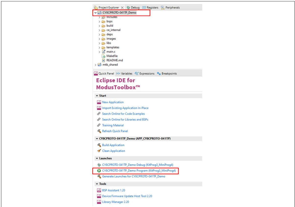
**Figure 16** Building and programming the code example
