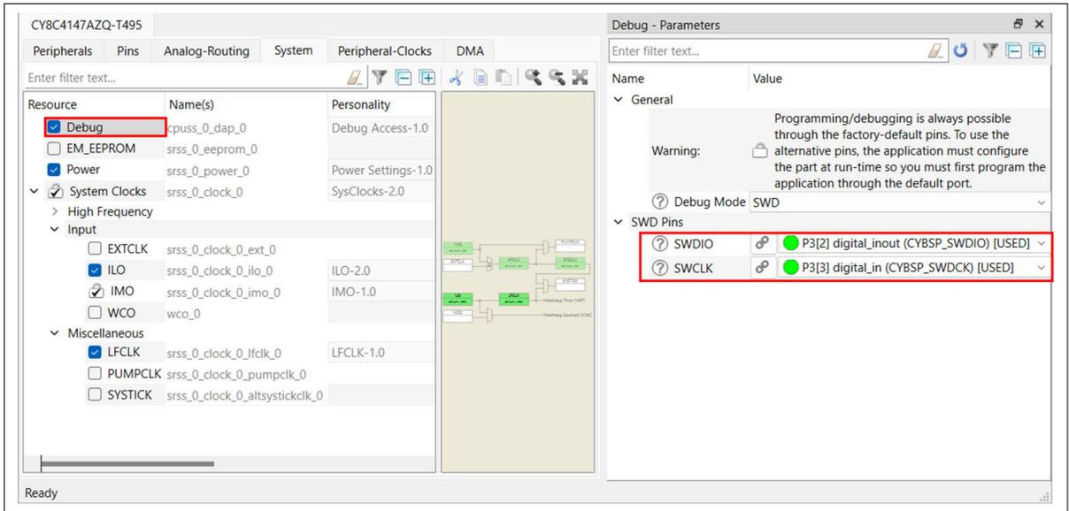
**Figure 17** Enabling Debug in the Device Configurator
