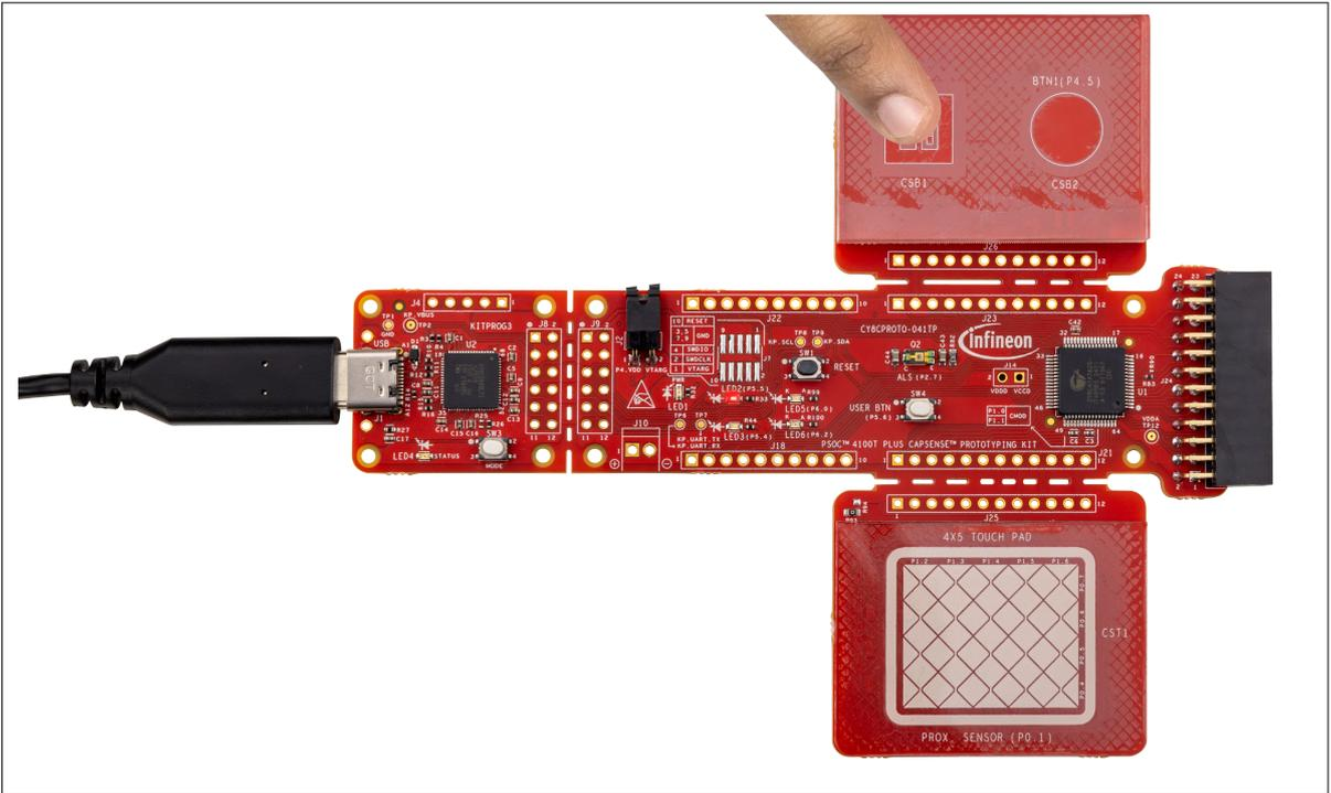
**Figure 8 CAPSENSE™ CSX button operation with LED indication**
