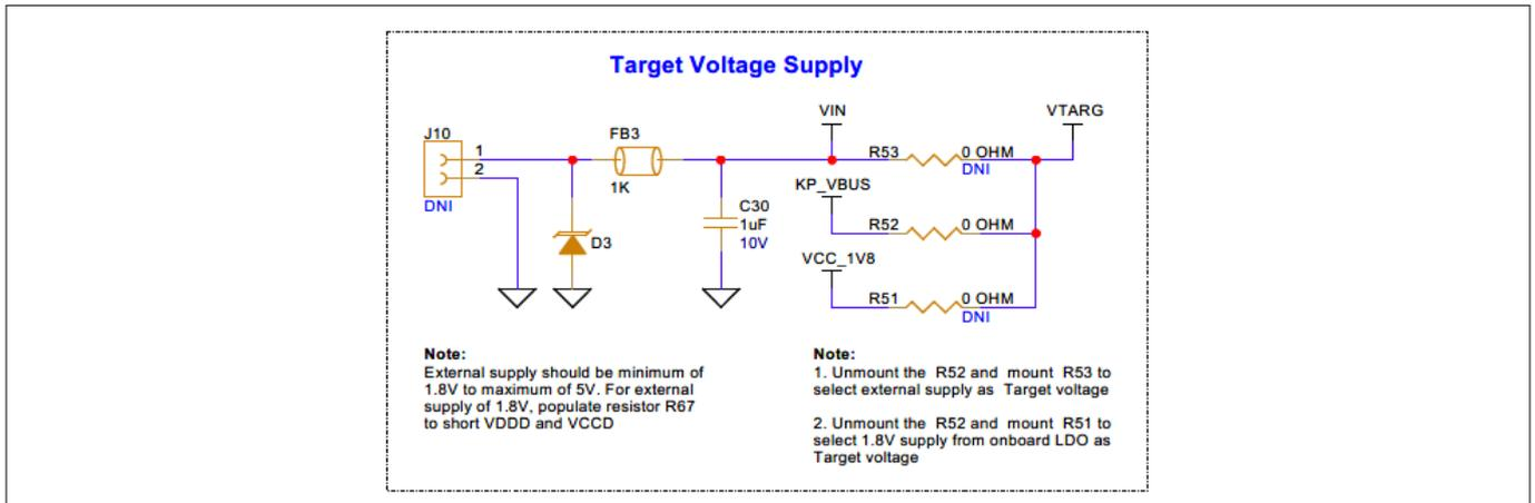
**Figure 34** External power supply input (J10) schematic
