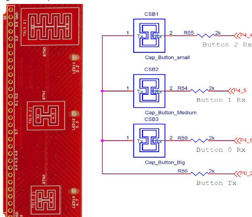
**Note:** Touching CapSense buttons and slider for about 2 sec will auto-reset the sensor, turning off LEDs. This is due to the auto-reset feature enabled in CapSense component for the Code example provided with the kit.
