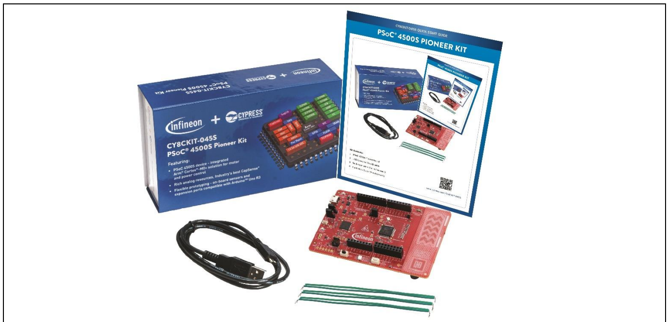
Figure 1 CY8CKIT-045S PSoC 4500S Pioneer Kit Contents
