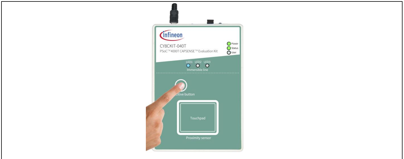
Figure 6 CAPSENSE™ button operation with LED indication
