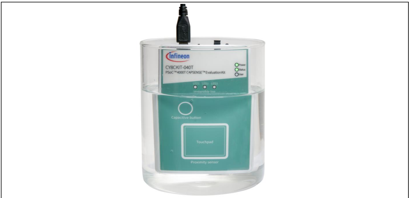
Figure 9 Immersing the kit inside water (up to immersible line)
