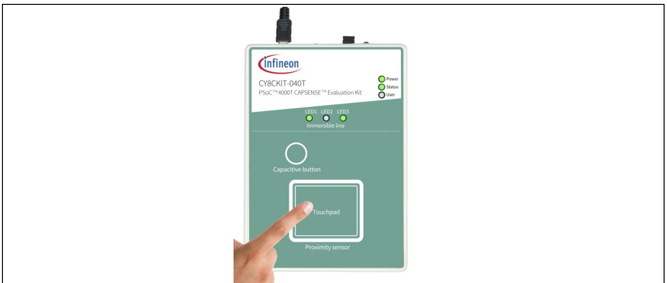
Figure 7 Capacitive touchpad operation with LED indication
