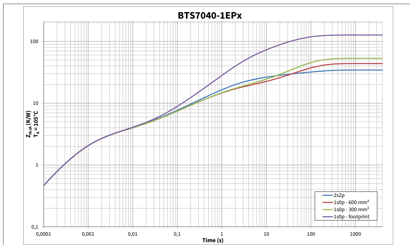
Figure 9 Typical Thermal Impedance. PCB setup according Chapter 4.4.1
