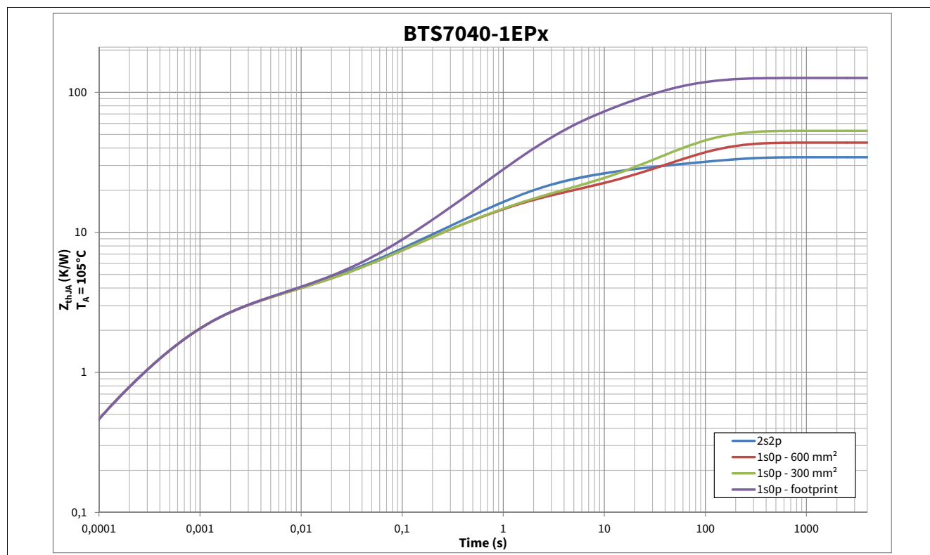
Figure 9 Typical Thermal Impedance. PCB setup according Chapter 4.4.1
