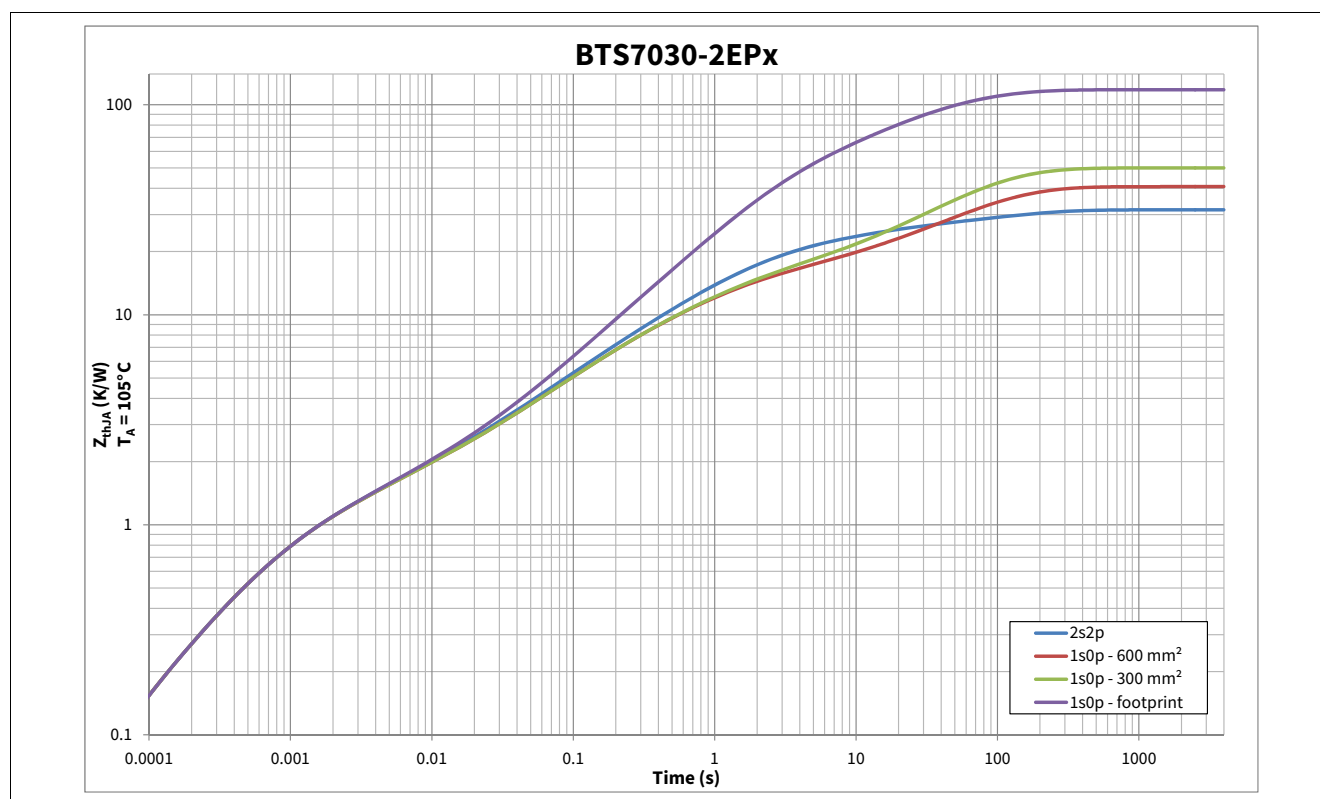
Figure 9 Typical Thermal Impedance. PCB setup according Chapter 4.4.1
