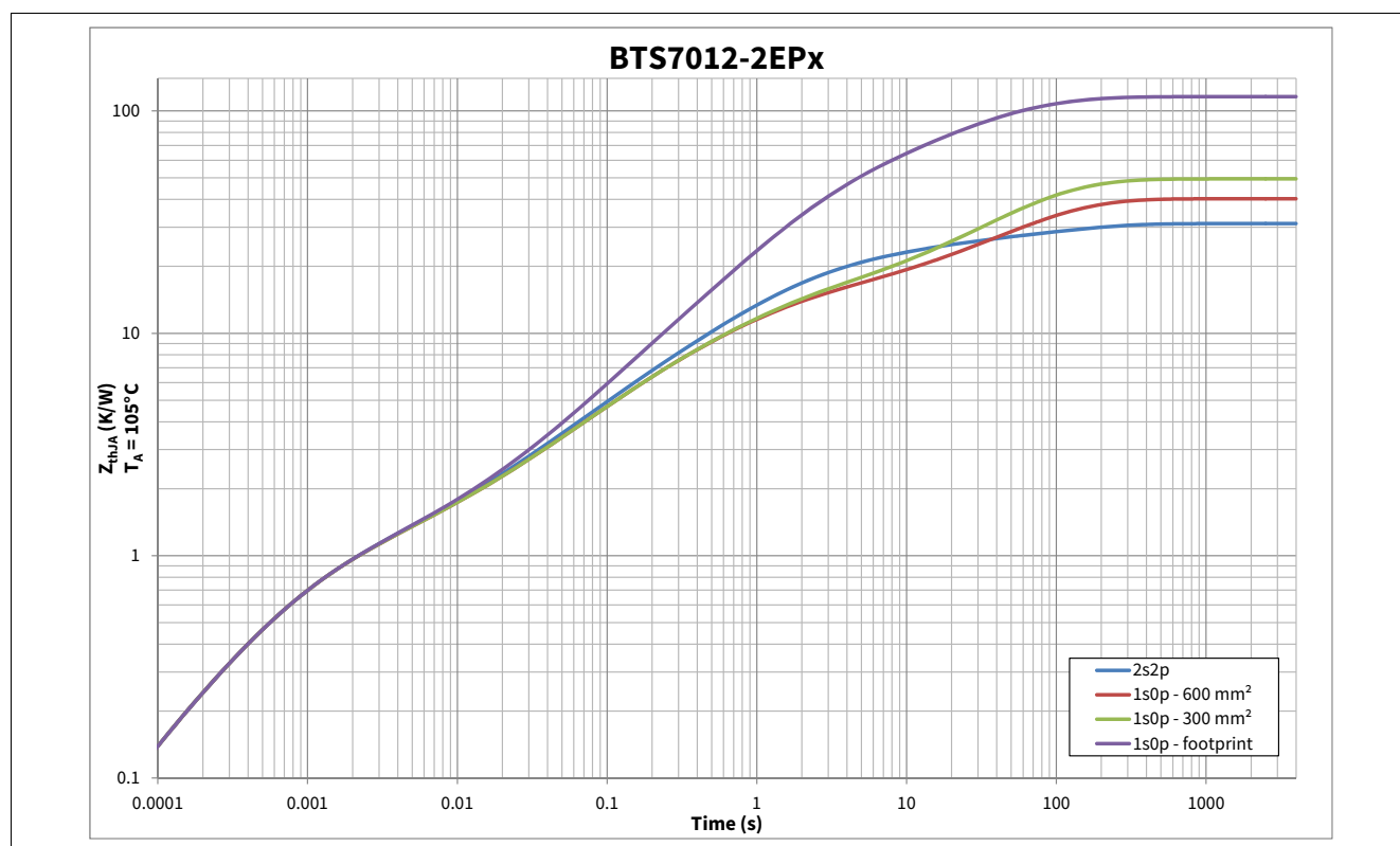
Figure 9 Typical Thermal Impedance. PCB setup according Chapter 4.4.1
