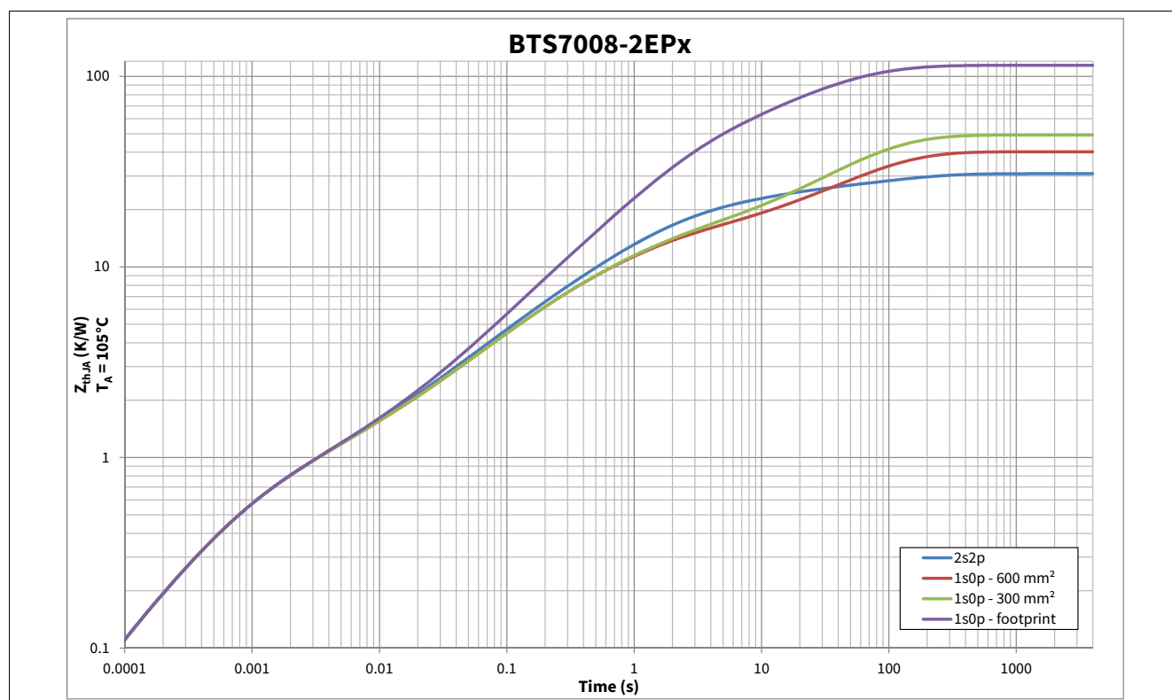
Figure 9 Typical Thermal Impedance. PCB setup according Chapter 4.4.1
