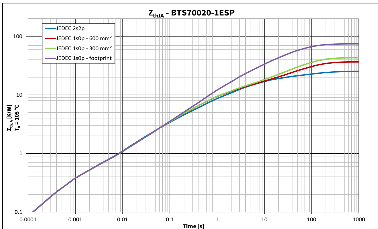
Figure 9 Typical Thermal Impedance. PCB setup according Chapter 4.4.1
