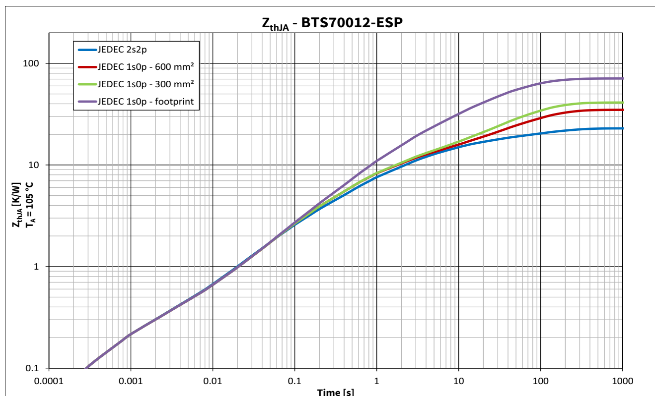
Figure 9 Typical Thermal Impedance. PCB setup according Chapter 4.4.1
