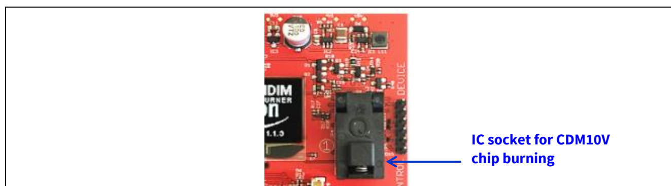
Figure 23 IC socket on the programming board for CDM10V chip burning
