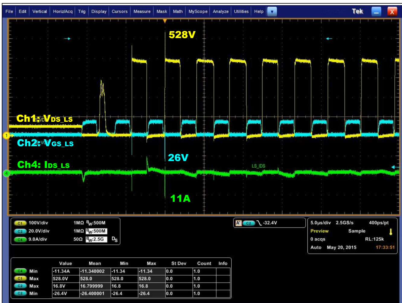
Figure 13 Hard commutation during burst mode operation, V_{DS\_pk} , V_{GS\_max/min} and I_{RRM}
