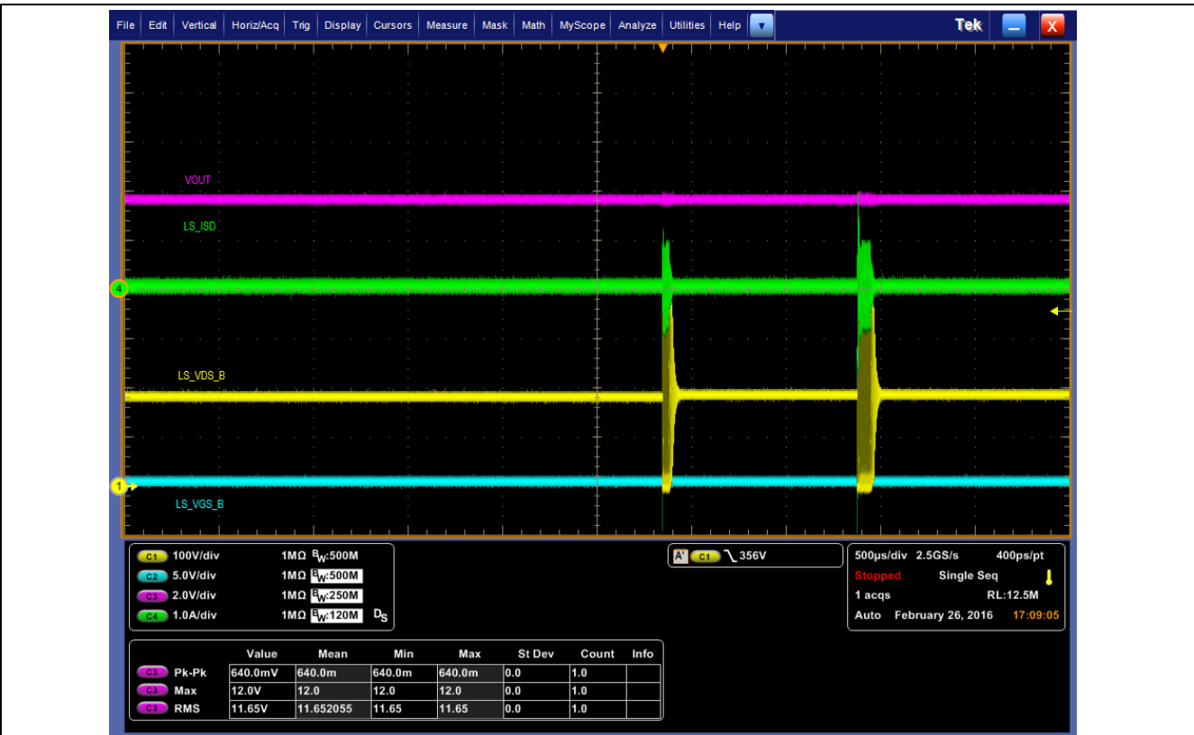
Figure 39 Burst mode operation at no-load and very light load condition with XMC4200
