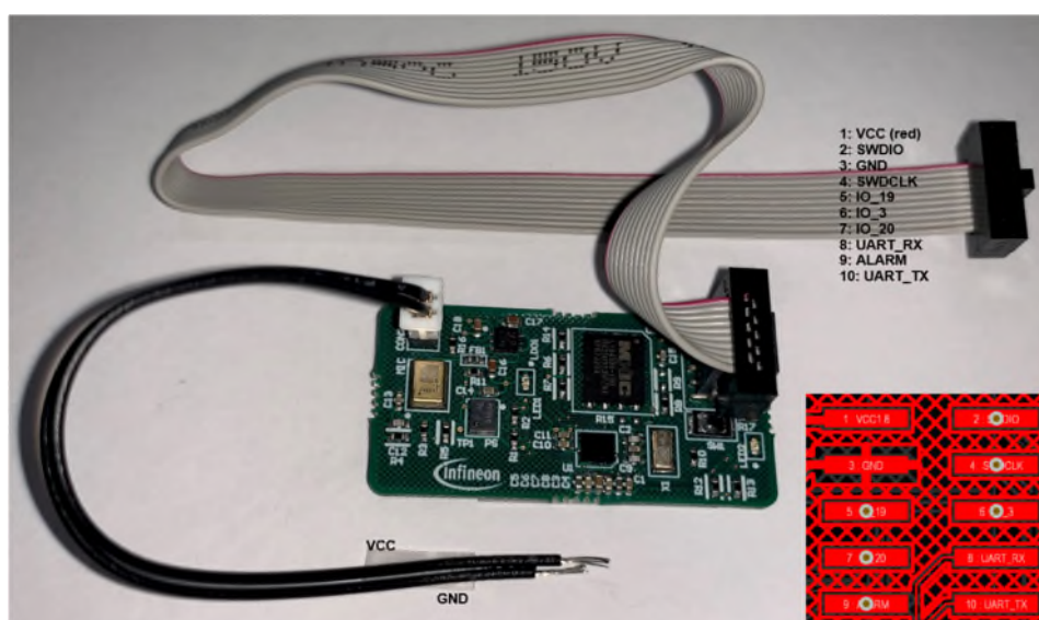
Figure 2 MicroIAS form-factor board connections
