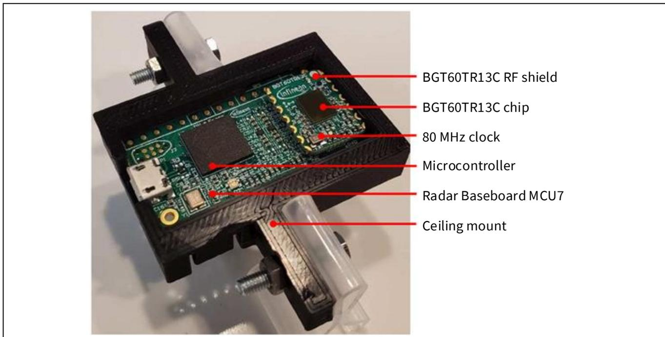
**Figure 2** DEMO BGT60TR13C board with ceiling mount
