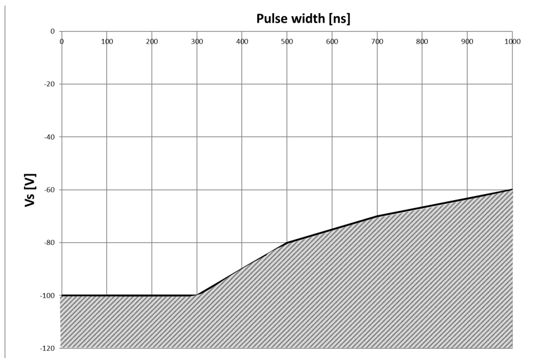
Figure 13 Negative transient voltage SOA on VS pin for 2ED2304S06F @ V_{BS}=15 V
