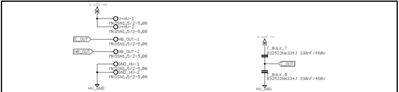
Figure 4-1: HV supply input and DC-Link capacitors
