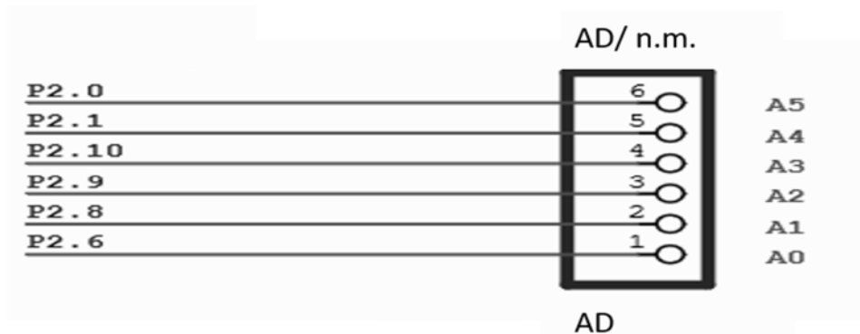
Figure 4 Analog input AD connector
