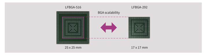
> LFBGA-292 and LFBGA-516 are ball compatible so that customers can build one PCB for both packages
