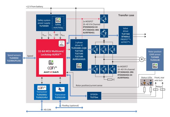
In Four-Wheel Drive (4WD) and All-Wheel Drive (AWD) vehicles, the transfer case is the part of the drivetrain responsible for the transfer of torque from the transmission to the front and rear wheels. The market now demands increased performance to drive BLDC motors and ever-greater functional safety requirements. AURIX<sup>™</sup> has the state-of-the-art safety features required to enable systems to achieve ASIL-D, the highest safety level.
