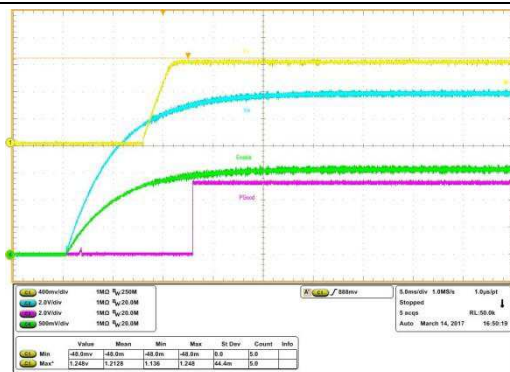
Start up at 16 A Load Ch1: V_{out} , Ch2: PV_{in} , Ch3: P_{Good} , Ch4: Enable
