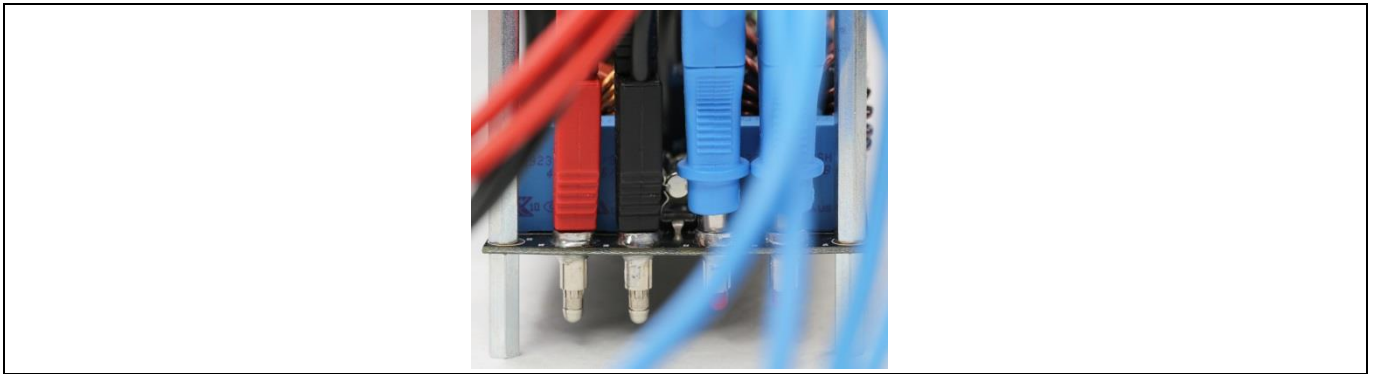
Figure 20 Wiring with force and sense wires for accurate efficiency measurements
