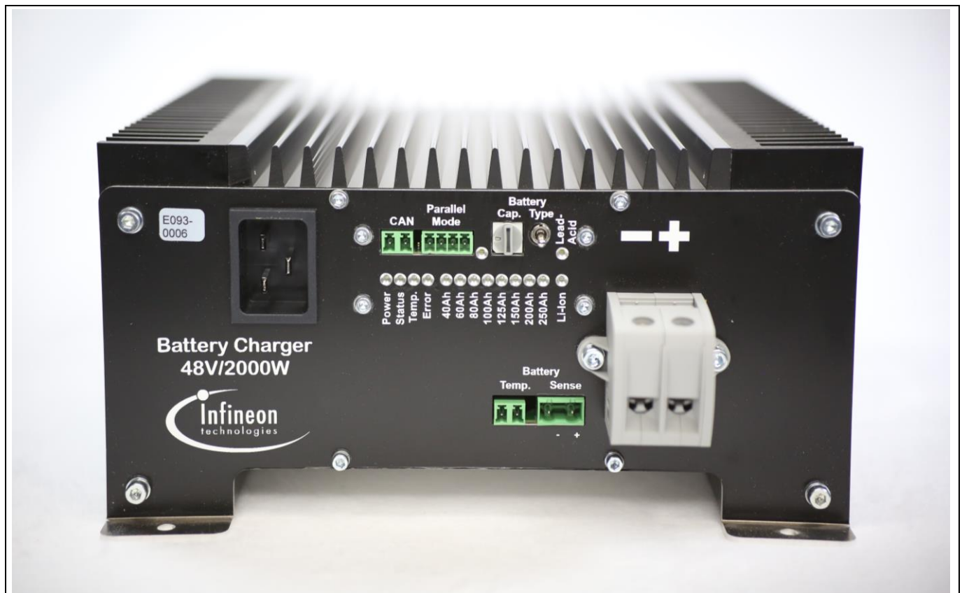
Figure 1 Front panel of the industrial battery charger
