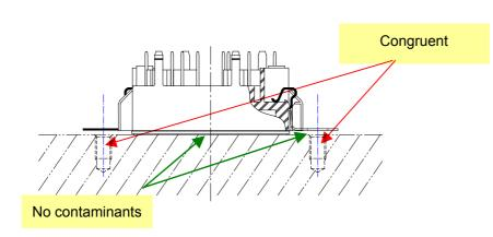
In order to position the module on the heat sink correctly a three pointstop pin on the heat sink is recommended.
