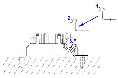
3. Soldering the module into the PCB
