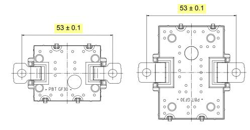
Note: If the module is soldered first into the circuit board or if a subsequent disassembly of the module is desired, appropriate sized through holes must be provided in the PCB (hole size depends on screwdriver or screw head diameter / washer).
