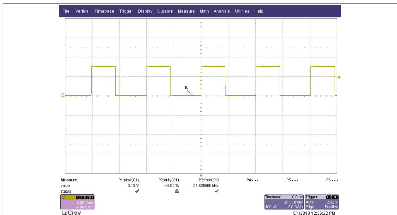
Figure 5 Onboard pulse-signal generator output (C1: IN)
