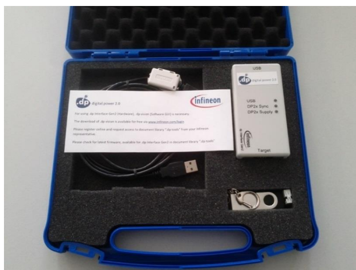
Figure 2 .dp Interface Gen2 Programming Kit Contents
