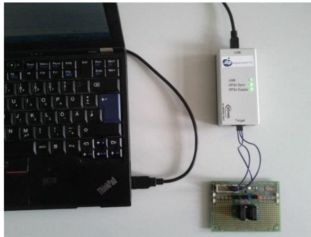
Figure 3 Interface Gen2 Box Connections to a PC and OTP Programming Board
