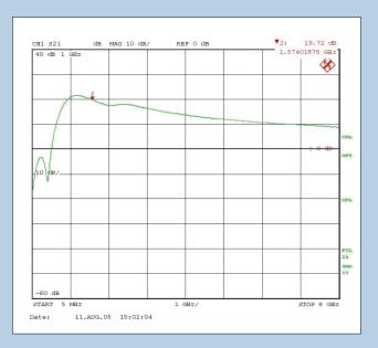
The picture left is the gain curve of BFP740F high Linearity GPS LNA. LNA has 20dB gain, 0.7dB noise figure, drawing 9mA from a 1.8 volt supply. 1.8 or 3.0V operation is possible with a single resistor value change. 10 external elements are used. Amplifier is unconditionally stable, e.g. k > 1,  $B_1 > 0$ . For more information please see application note AN117.
