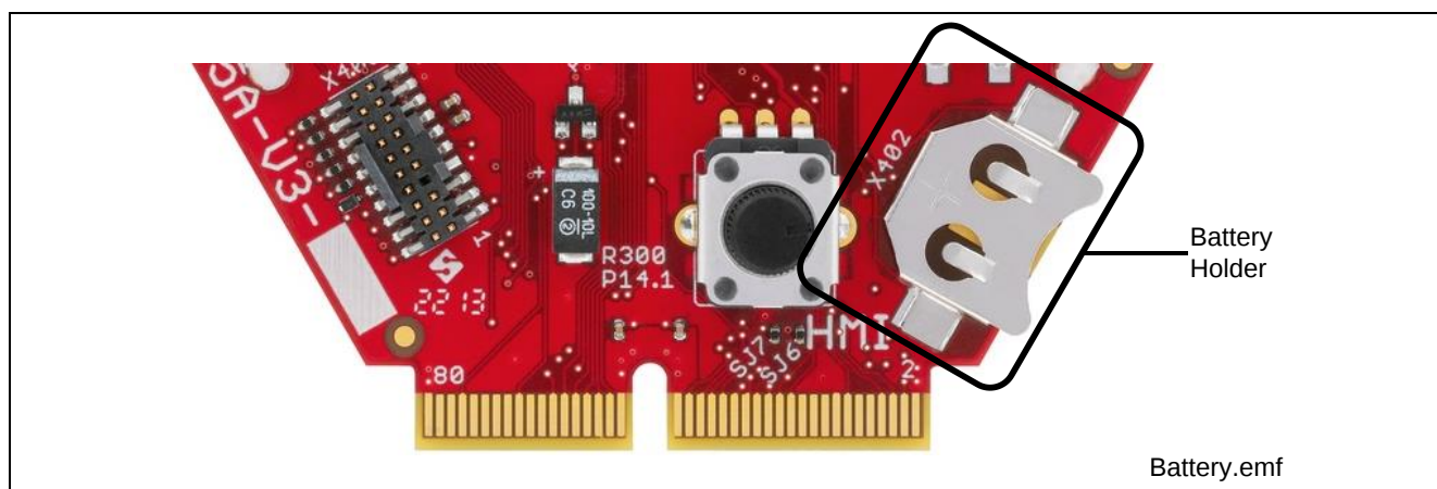
Figure 5 Battery (VBAT Supply)
