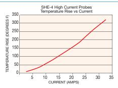
1. For SH-4 Series only 2. Smiths Interconnect's current ratings are defined as the maximum current at which the temperature rise of the probe does not exceed 144°F (80°C) for a single probe in free air at ambient temperature for one hour. Dimensions are in inches (mm) | All specifications are subject to change
