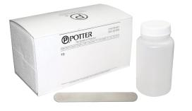
This kit is designed to conform to the requirements of NFPA 25, 2002, 13.2.1.2 requiring testing for MIC if slime or tubercles are discovered in an internal inspection. The test involves removing some of the slime, deposit, scale, tubercles, mounds, etc. and sending them to Potter for microbiologically influenced corrosion (MIC) analysis.
