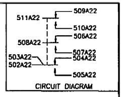
SWITCH CURRENT LEVELS SHALL NOT BE MORE THAN 100 MILLIAMPS @ 28 VDC PRINT CIRCUIT DAGRAM, CATALOG LISTING, DATE CODE AND NAVAIR PART NUMBER
