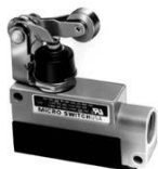
Enclosed Switches Series BZG/BZH: Top Roller Arm Actuator, Adjustable with Steel Roller; 1NC 1NO SPDT Snap Action; 1/2 in - 14NPT conduit
